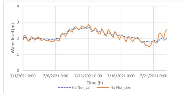
Fig. 11. Validation of water level at Ha Noi station, 2021
